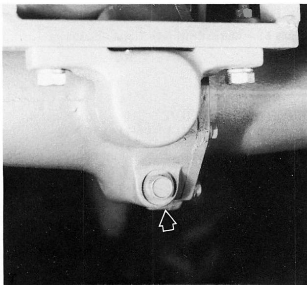
Figure 63 — Front Axle Differential Drain Plug
