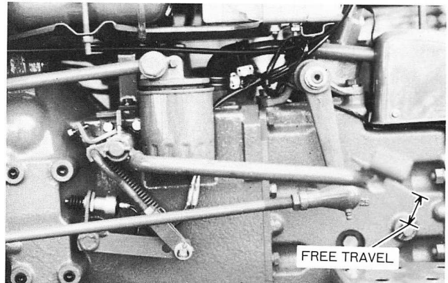
Figure 61 – Clutch Pedal Free Travel Adjustment
